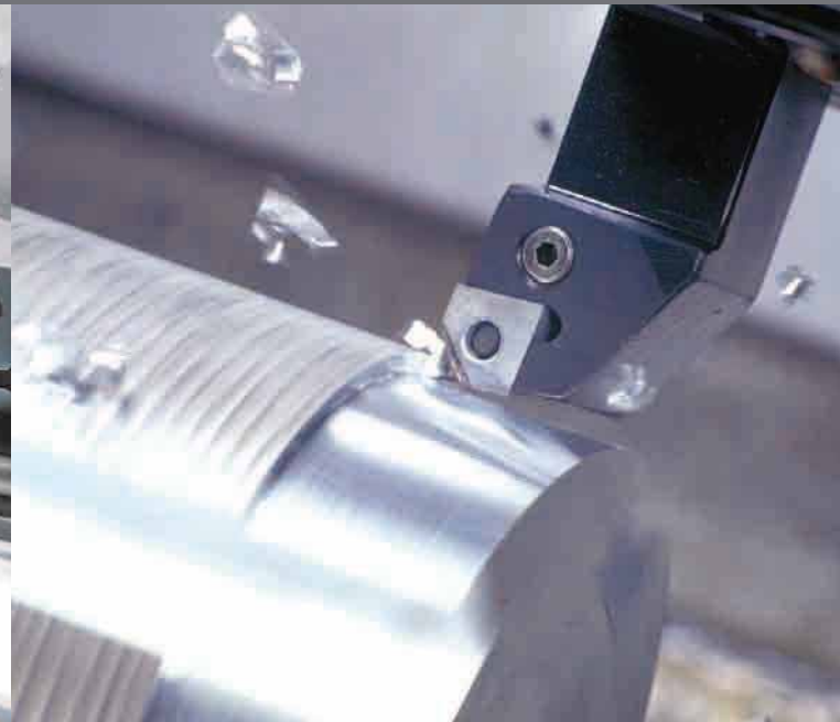
使用SumiDia刀片进行铝断续切削 Interrupted Aluminum cutting by SUMIDIA inserts
