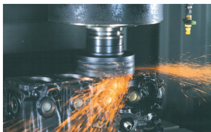
使用住友CBN刀片进行铸铁切削 Cast iron cutting by SUMIBORON inserts
